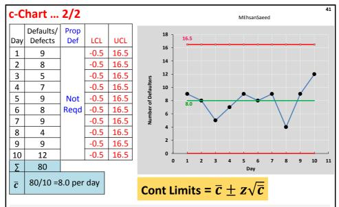
Here, the SD  $\sqrt{\bar{c}}$  is constant .: LCL &UCL for all observations are also constant, giving straight lines  $\bar{c}=\frac{80}{10}=8.0$ , z=3
